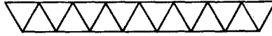
FIG. 4. A structure which resists bending, constructed from links which resist both compression and extension. We use this structure in the two-dimensional representation of a disk for an artificial valve.
